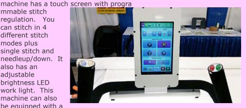
Nolting also has a commercial machine with the Intellistitch Equalizer stitch regulator, standard speed control, needle up/down, and fixed handles in the front & rear. This machine can also be equipped with a computer.
